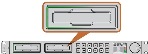
SSD slots on HyperDeck Studio models have rotating LEDs to show the unit is in playback mode.
