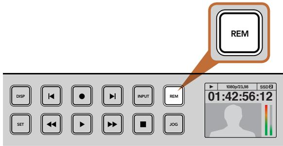
Press the REM button on HyperDeck Studio models to enable RS-422 deck control.
