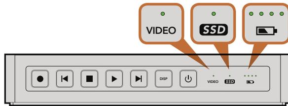
Status indicators on HyperDeck Shuttle tell you whether your SSD is formatted correctly, whether a video signal is detected and how much battery power is left.
