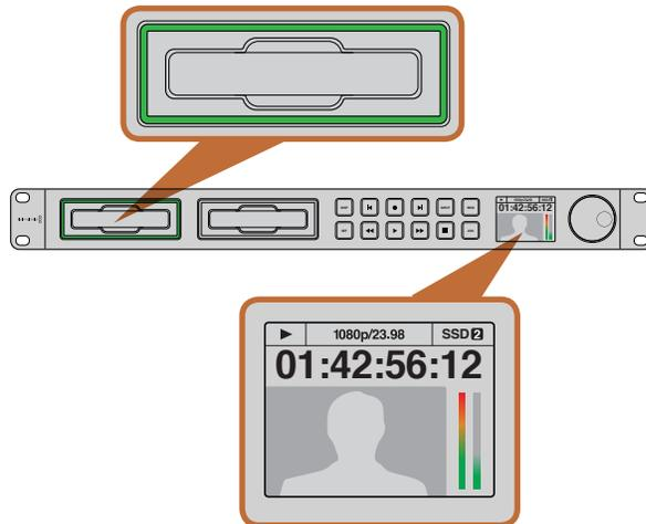
The SSD slots on HyperDeck Studio models indicate if an SSD is formatted correctly and whether the unit is in recording or playback mode. The LCD on HyperDeck Studio models shows your video as well as status information.
