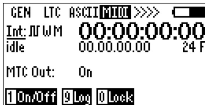
Changes the status of the midi timecode (MTC) generator. In this first software version the MTC generator is locked to the main timecode generator at all times. In future software the MTC in will be activated as well as the possibility to run the MTC generator at a different frame rate from the main LTC generator allowing a gearbox function.
