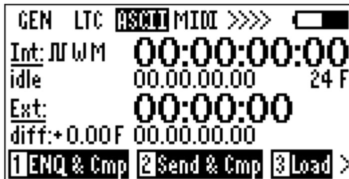
In this menu timecode can be sent, received and compared using the Aaton ASCII protocol. This protocol sends and receives ASCII messages about timecode and is not a continuous data transfer. The Ambient IR interface will also use this protocol to communicate with external Timecode equipment without cables,
