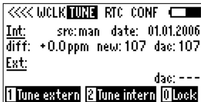
This menu is used to tune (calibrate) other Clockit devices or for the Controller to calibrate its reference oscillator to an external source. The internal reference can be tuned to + - 10ppm with a resolution of 0.15 ppm per digit. The tuning number DAC is shown on the display as well as recent tuning history. The tuning protocol uses an ASCII format connected as cable or through infrared. The tuning process may have
